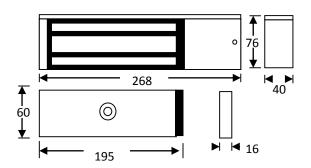
Standard single unmonitored magnetic lock, designed for indoor applications where 545kg holding force is required. This model includes door status monitoring contacts to monitor the door position (open or closed).
