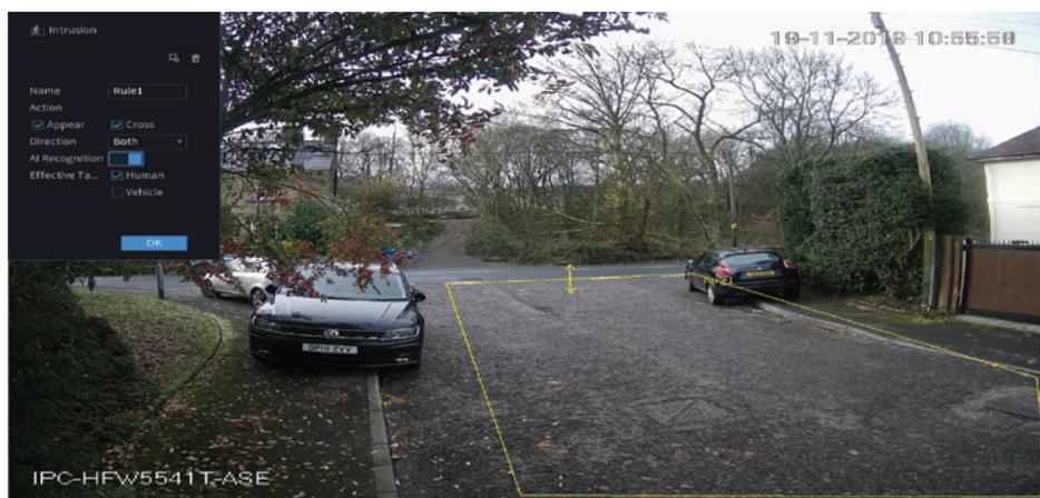
Rules can be created using the left mouse button to draw Tripwire or Intrusion lines on the image in the area of interest. In the top left window, the direction of travel can also be selected. Once the rule is configured, click **Ok**
