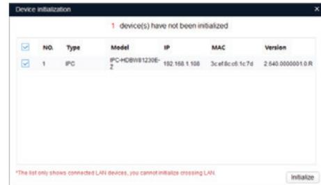
Enter the new password to be used for the camera and an email address for password recovery. Set P/N to P and click next to continue
