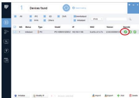
Enter the new IP address the camera is to be set to
