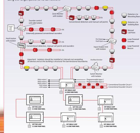
This diagram is provided for illustration purposes only and you should always refer to the relevant XFP panel/device instructions as appropriate before installation. Note that the descriptions and availability of the devices shown may not be applicable to all manufacturer's protocols.
